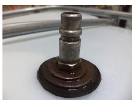
FIG. 2 Water Inlet Quick Connect Fitting
