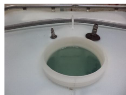
FIG. 3 Quick Connect Fitting Locations
