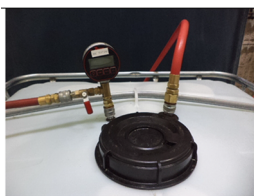
FIG. 4 Fitting and Closure Final Assembly
