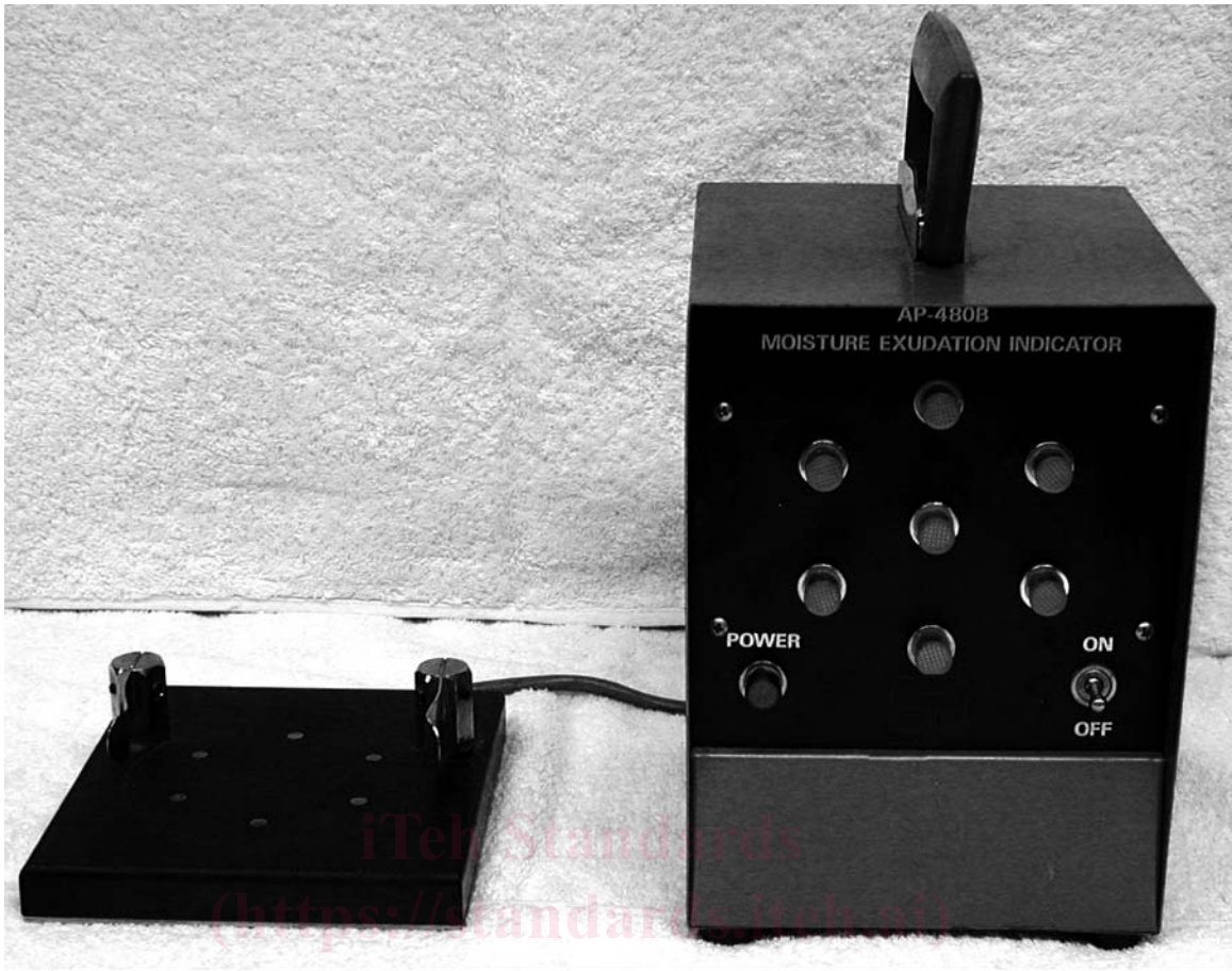
FIG. 4 Circular Exudation-Indicator Device
