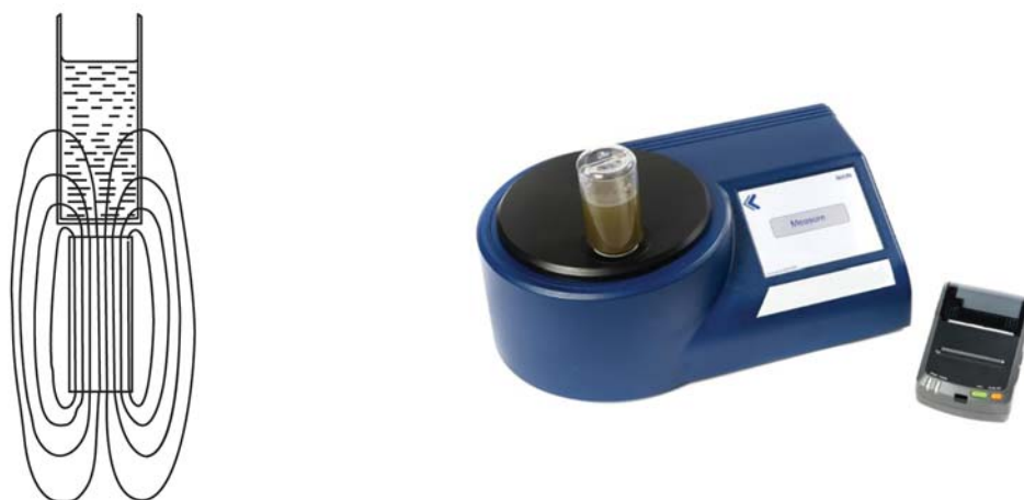
FIG. 1 Principle of PQ Magnetometry (left) and a Modern Instrument (right)
