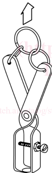
FIG. 5 Tension Test Adapter/Clamp
