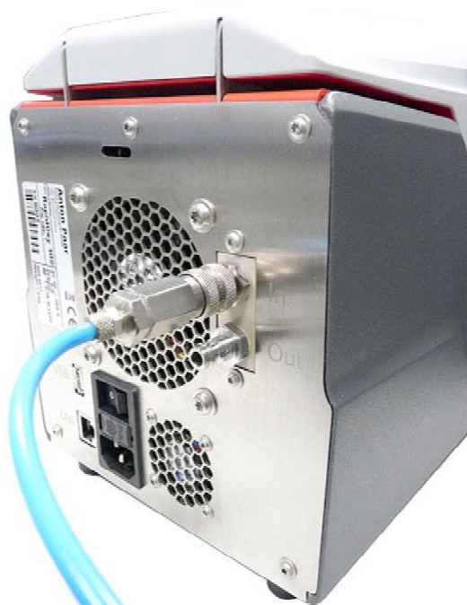
FIG. 2 Example of Rear View of Instrument with Oxygen Inlet and Outlet Valve
