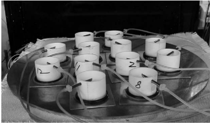
FIG. 3 Test Coupons on Hot Plate
