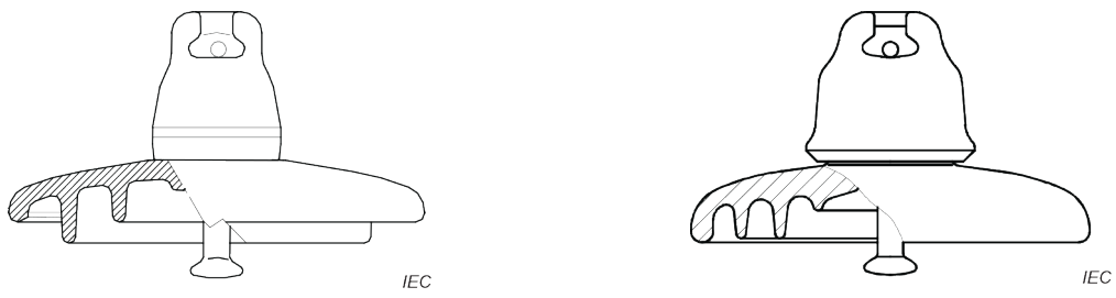
Figure 1 – Typical "standard" profile
