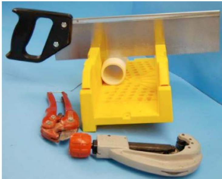
FIG. 5 Cut Pipe Square
