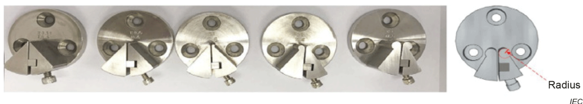
Figure 5 – Flexibility folding jigs (from the left, folding radius r is 1,0 mm, 2,0 mm, 3,0 mm, 4,0 mm, 5,0 mm and 10,0 mm)
