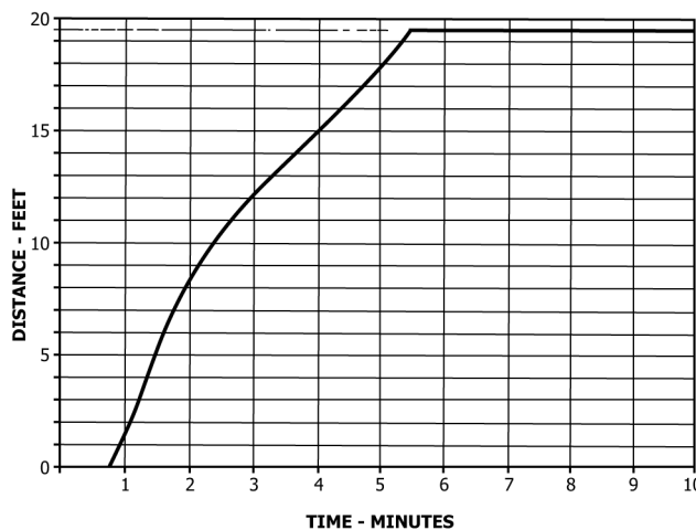
FIG. 7 Representative Time-Distance Curve for Flame Spread of Red Oak
