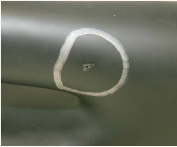
FIG. 6 Breakdown (Dielectric Failure)
