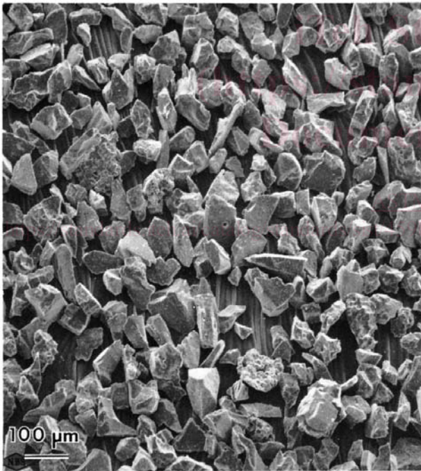
FIG. 3 Photomicrograph of 50 \mu\text{m} \text{Al}_2\text{O}_3 Particles Used in Inter-laboratory Testing
