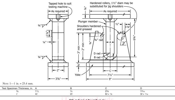
FIG. 1 Guided-Bend Test Jig
