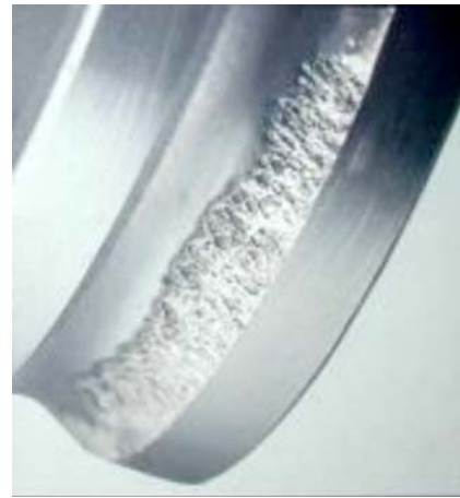
FIG. 2 Typical Bearing Spall
