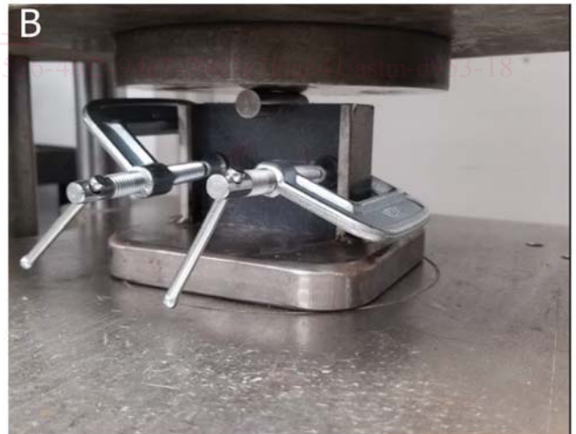
FIG. 5 Compression Loading Fixture for Procedure C (With Picture of Sample Under Pin-Bearing Load)
