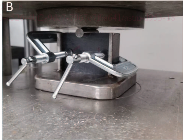
FIG. 5 Compression Loading Fixture for Procedure C (With Picture of Sample Under Pin-Bearing Load)
