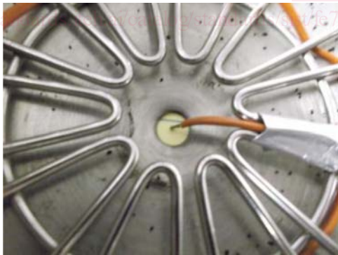
FIG. 4 Thermocouple Location in Coffee Filter Basket for Monitoring Batch (Type II) Brewer Dispensing Temperature
