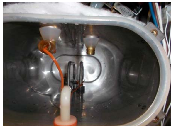
FIG. 1 Thermocouple Location for Monitoring Internal Water Tank Temperature
