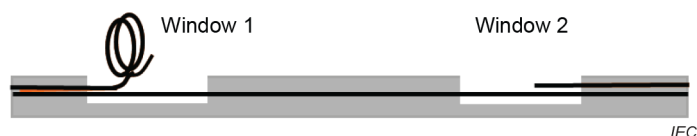
Figure 37 – Concept of straight midspan access
