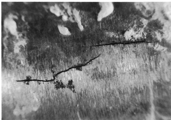
FIG. 2 Typical External Stress Corrosion Cracks (5× Magnification)
