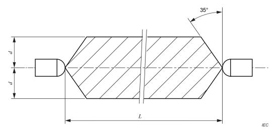
For type 4: d = 131 mm, L = 250 mm to 3 000 mm For type 3: d = 184 mm, L = 375 mm to 3 000 mm For type 2: d = 262 mm, L = 500 mm to 3 000 mm
