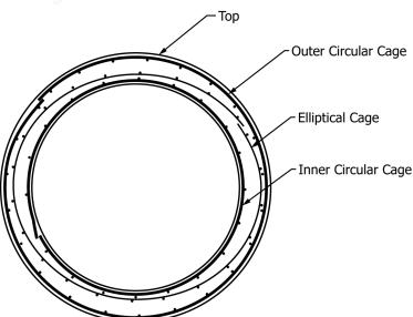
Note 1—The total reinforcement area of the inner circular cage and the elliptical cage shall not be less than that specified for the inner cage in Tables 1-5.
