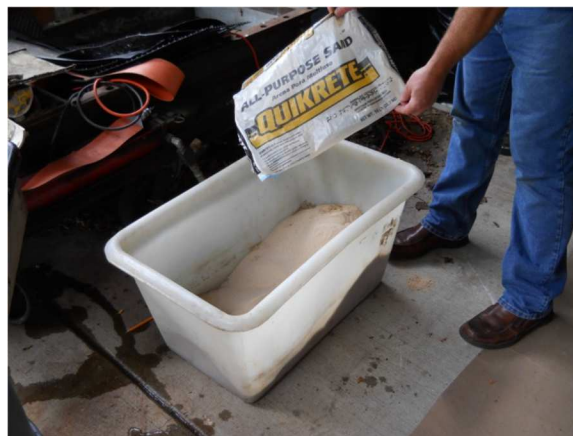
FIG. X1.1 Sand Placed in Base of Tub
