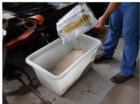
FIG. X1.1 Sand Placed in Base of Tub
