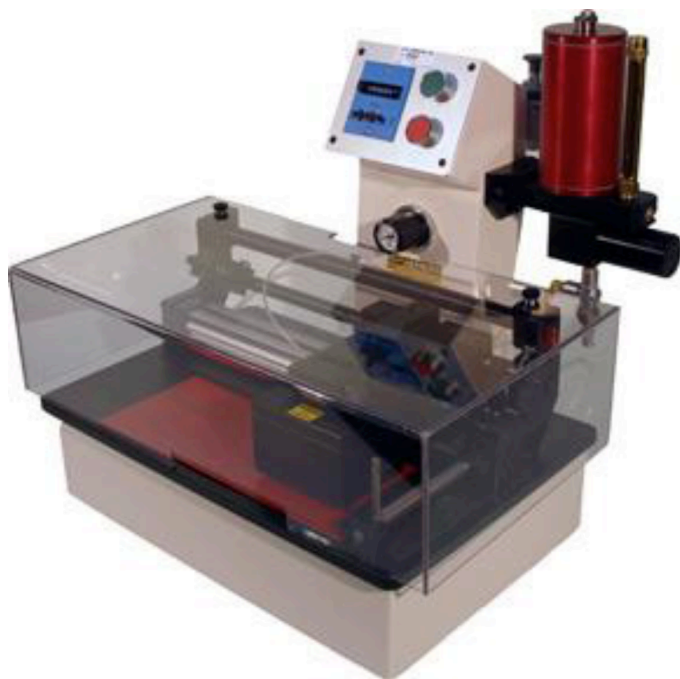
FIG. 1 Example of a Mechanical Rubbing Machine
