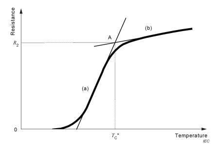
The cryogenic resistance,  $R_2$  is determined by the intersection,  $A_r$  of two straight lines (a) and (b) at temperature  $T_c$ \*. (standards.iteh.ai)
