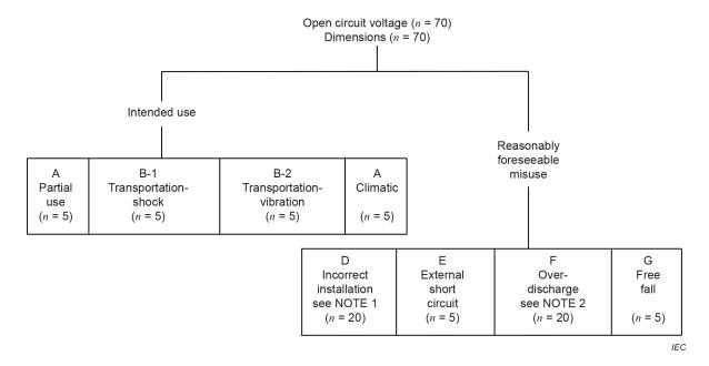
NOTE 1 Four batteries connected in series with one of the four batteries reversed (5 sets).
