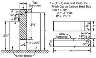
Shear Blocks shall be Bolted Firmly Together against Filler Piece which Provide Space 0.005" Wider than t of Specimen
