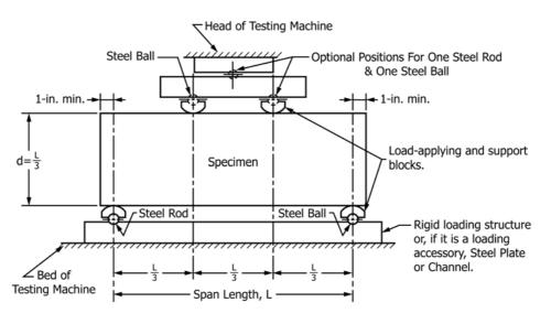
Note 1—This apparatus may be used inverted. If the testing machine applies a force through a spherically sealed head, the center pivot may be omitted, provided one load-applying block pivots on a rod and the other on a ball. Note 2—1 in. = 25.4 mm.
