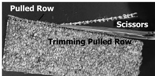
FIG. 1 Photograph of Trimming the Edge of a Pulled Tufted Row of Yarn
