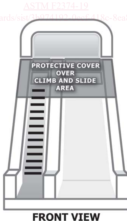
FIG. 8 Protective Cover Over Slide and Climb Areas
