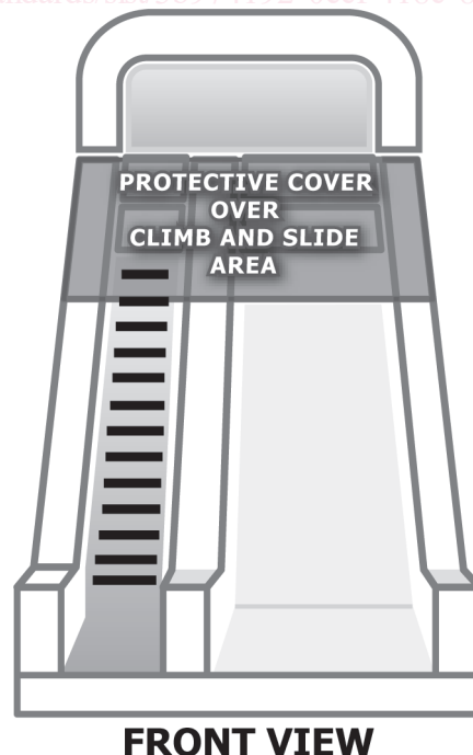
FIG. 8 Protective Cover Over Slide and Climb Areas
