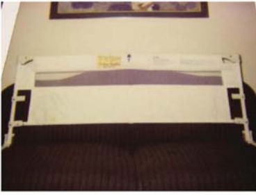
Center horizontal structural component is omitted consequently the fabric does not engage the center structural component.
