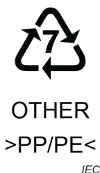
Figure 2 – Marking of polypropylene-polyethylene copolymer battery components
