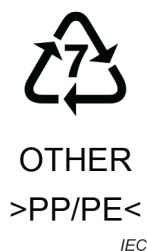
Figure 2 – Marking of polypropylene-polyethylene copolymer battery components
