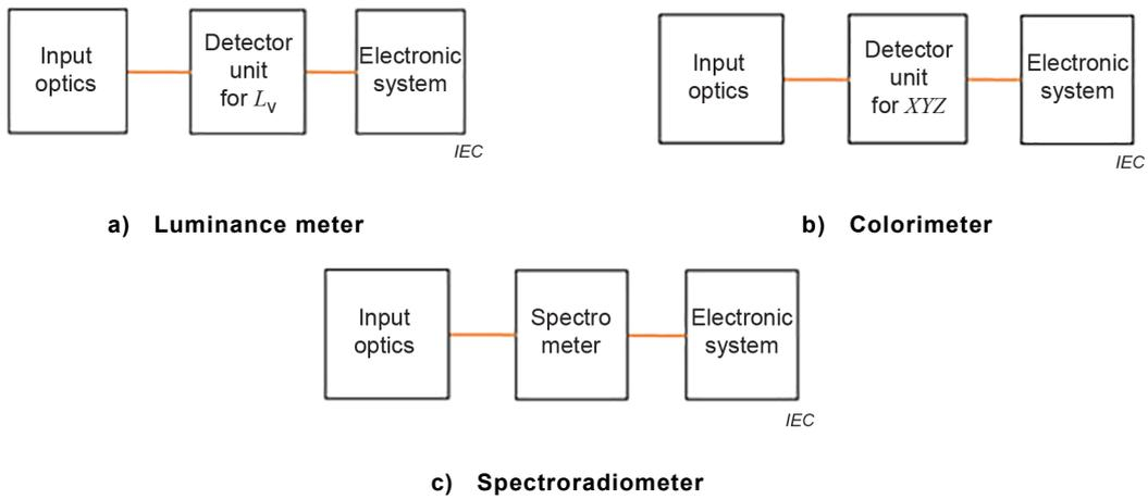
Figure 1 – Block diagrams of three types of LMDs
