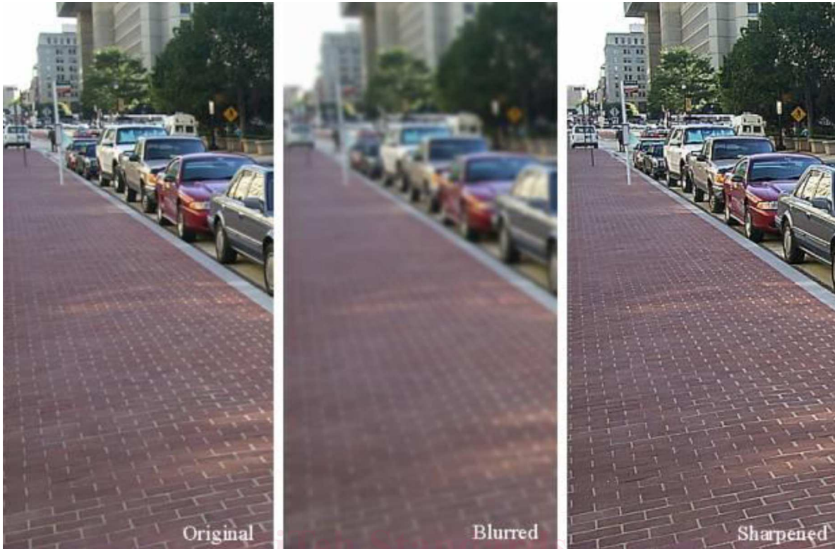
FIG. 1 This Example Illustrates the Effects of Linear Filtering—Left: Original Image, Middle: Blurred Image, and Right: Sharpened Image
