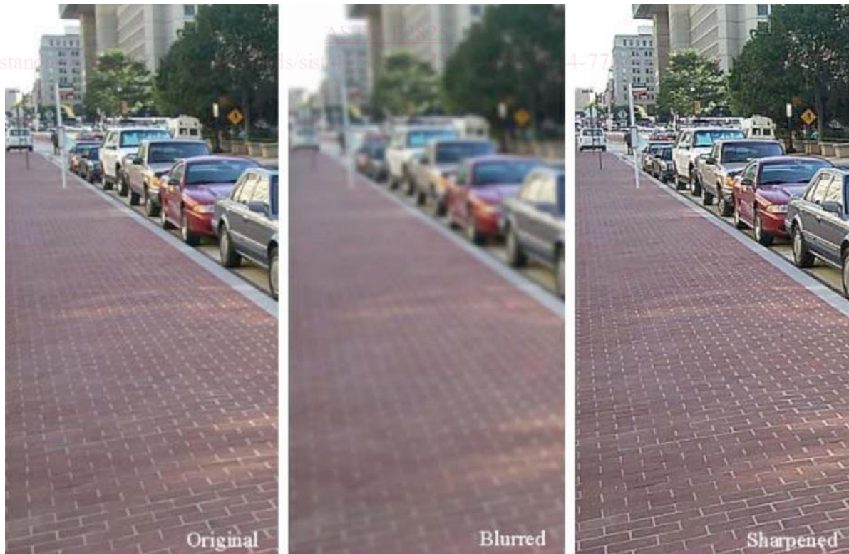
FIG. 1 This Example Illustrates the Effects of Linear Filtering—Left: Original Image, Middle: Blurred Image, and Right: Sharpened Image
