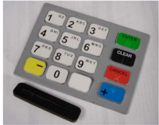
FIG. 14 Example of Keypad Overlay
