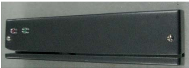
FIG. 5 Example of a Custom Skimmer (Door)
