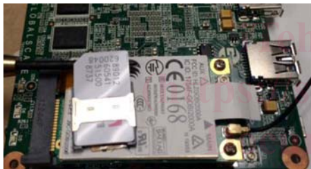
FIG. 6 Example of a Cellular Enabled Skimmer
