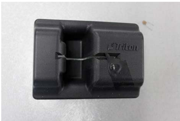
FIG. 10 Front View of a Skimmer Using Separate Boards for Capturing Track Data and PINs
