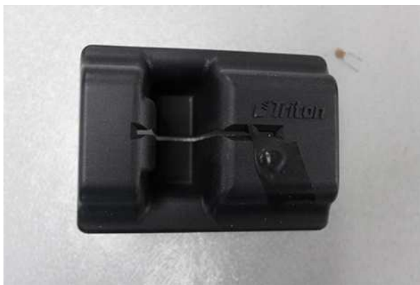
FIG. 10 Front View of a Skimmer Using Separate Boards for Capturing Track Tata and PINs
