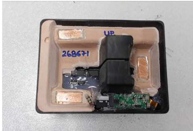
FIG. 11 Rear View of a Skimmer Using Separate Boards for Capturing Track Data and PINs
