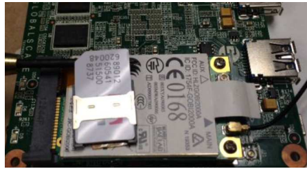
FIG. 6 Example of a Cellular Enabled Skimmer
