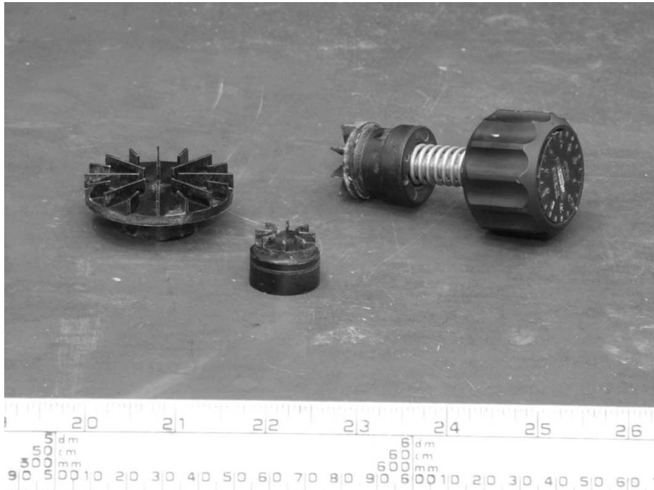
FIG. 1 Example of a Typical Torsional Shear Device with Standard (mid-size) Vane Attached, Along with Smaller and Larger Sized Vanes
