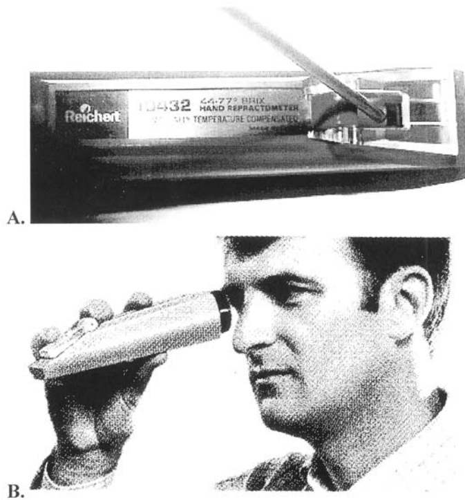
(A) Application of the aqueous polymer quenchant to the refractometer. (B) Visual reading of the refractometer scale to determine refractance value. FIG. 6 Typical Hand-Held Refractometer
