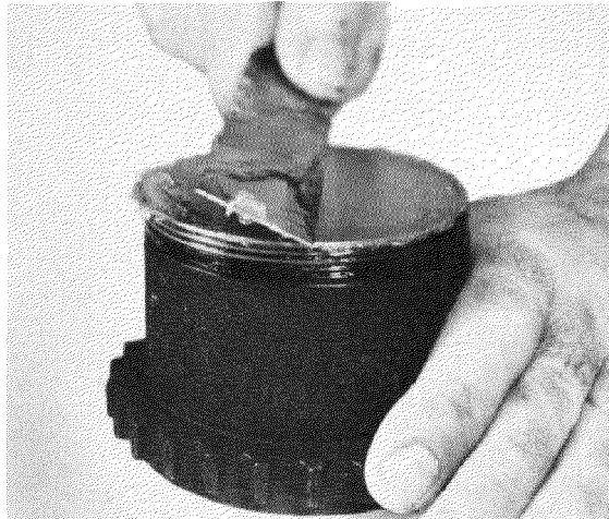
FIG. 2 Preparing Sample for Penetration Measurement
