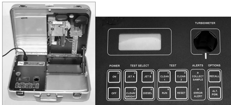
FIG. 2 Mark X Micro-Separometer and Control Panel
