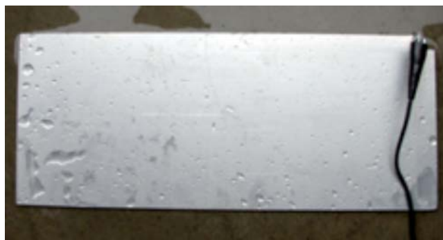
FIG. 6 Ground Connection Using a Metal Plate
