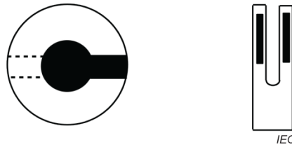
Figure 1 – Conceptual diagrams for sensor elements of BAW resonator type
