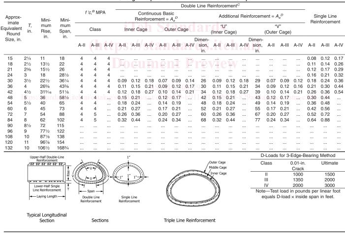
TABLE 1 Strength Requirements for Reinforced Concrete Pipe<sup>A</sup>
