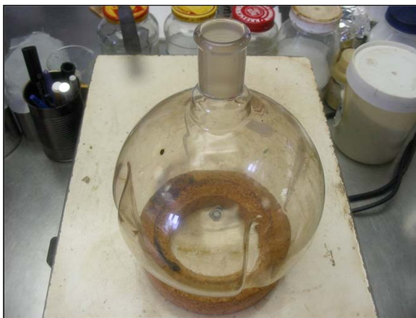
FIG. 3 Two-Liter Morton Flask on Cork Ring
