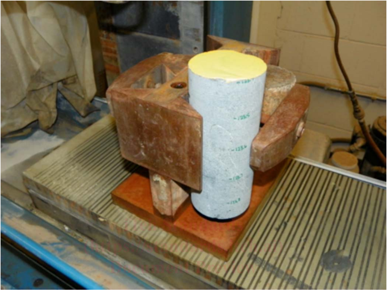
FIG. 3 One example of Holding Jig for Surface Grinder that can be Rotated and Grind Both Ends of up to Four Specimens (The adjacent short core is used as a spacer to fill unused specimen slot and yellow on top of specimen is placed prior to grinding for showing where grinding is occurring as the surface grinding progresses. Once lapping of the visible specimen end is completed the top half of the jig is unbolted and the section rotated so the opposing end of the specimen is now facing up and can be lapped as well.)
