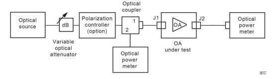
d) Measurement of total output power
