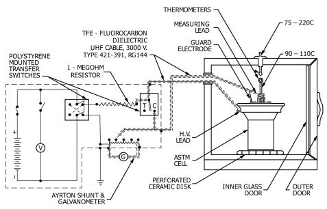
Note 1—For measurements of current less than  $10^{-9}$  A replace galvanometer and shunt with picoammeter.
